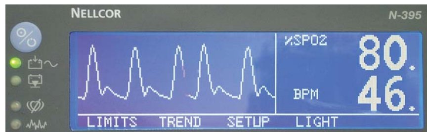
Figure 15. Photo of notched waveform at 45 bpm as displayed by Nellcor N-395 in response to input signal shown in figure 13. Notice that the waveform is distorted and the notch is well below midline.
