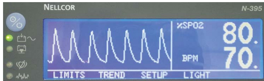
Figure 7. Photo of waveform at 70 bpm displayed by Nellcor N-395 in response to input signals shown in figure 5. Notice that the waveform is distorted and shows a curvature, which is not present in the input signal.
