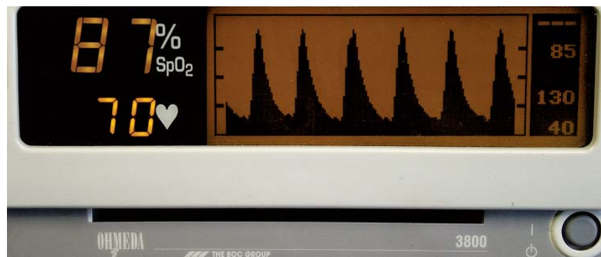
Figure 8. Photo of waveform at 70 bpm displayed by Datex-Ohmeda 3800 in response to input signals shown in figure 5. Notice that the waveform is distorted and shows a curvature, which is not present in the input signal.
