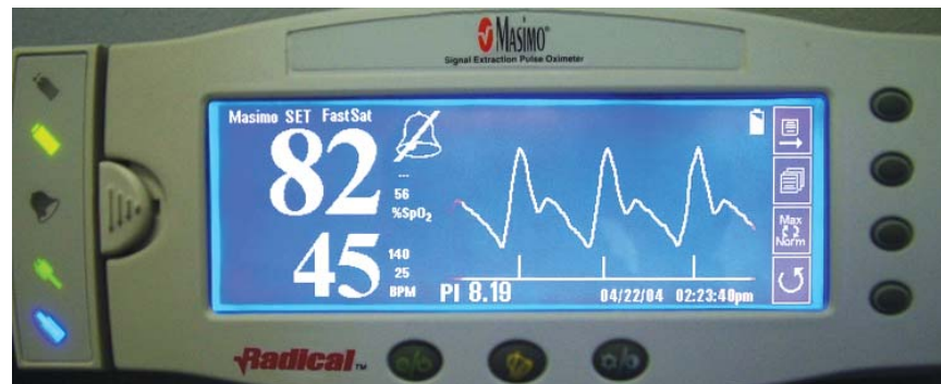
Figure 14. Photo of notched waveforms at 45 bpm as displayed by Masimo Radical in response to input signal shown in figure 13. Notice that the waveform integrity is preserved.
