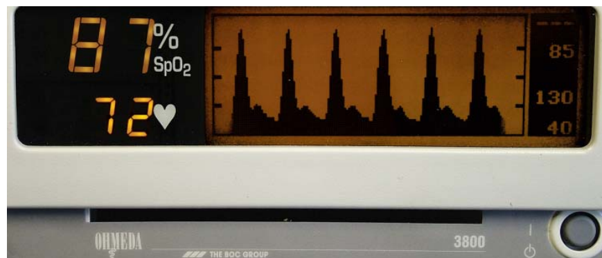
Figure 12. Photo of notched waveform at 72 bpm as displayed by Datex-Ohmeda 3800 in response to input shown in figure 9. Notice the distortion in waveform and the notch well below midline.
