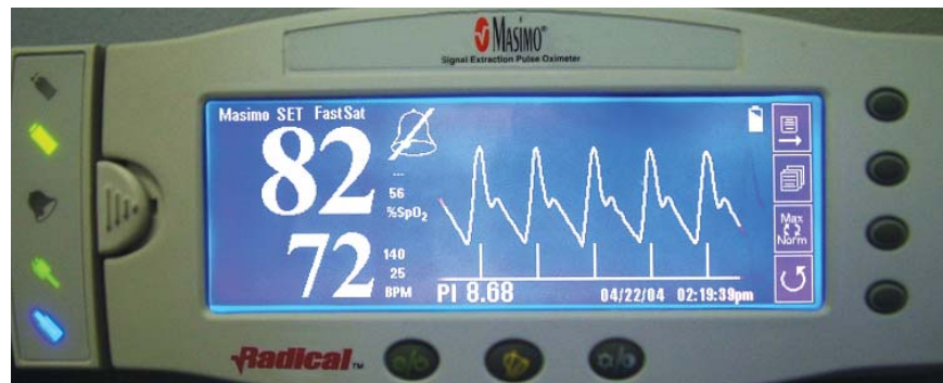
Figure 10. Photo of notched waveform at 72 bpm displayed by Masimo Radical in response to input signals shown in figure 9. Notice the notch appears at mid level and waveform integrity is excellent.
