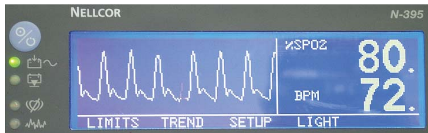
Figure 11. Photo of notched waveform at 72 bpm displayed by Nellcor N-395 in response to input signals shown in figure 9. Notice the distortion in waveform and the notch well below midline.
