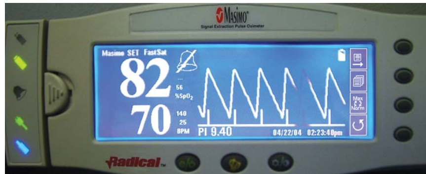
Figure 6. Photo of waveform at 70 bpm displayed by Masimo Radical in response to input signals shown in figure 5. Notice that the waveform integrity is maintained.
